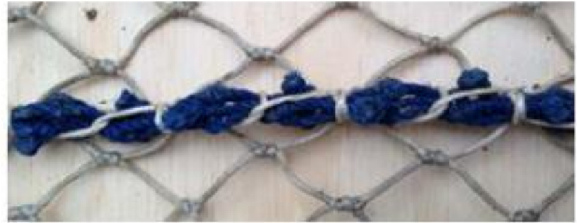
Figure 5. Bracing rope installed at the hanging ratio of 0.707 along the longitudinal centre line of the trawl to increase the stain transfer to the tongues.
